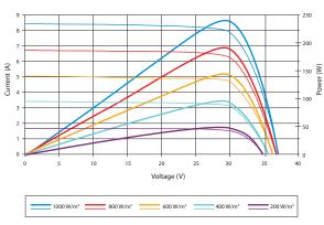
Exellent performance under weak light conditions: at an irradiation intensity of 200 W/m² (AM 1.5, 25 °C), 96% or higher of the STC efficiency (1000 W/m²) is achieved
